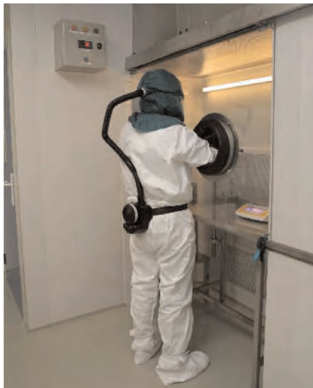
Figure 2. SCF - processed powder from a particle-generation SCF equipment harvesting in a laminar hood inside a clean room. (Courtesy SEPAREX)
