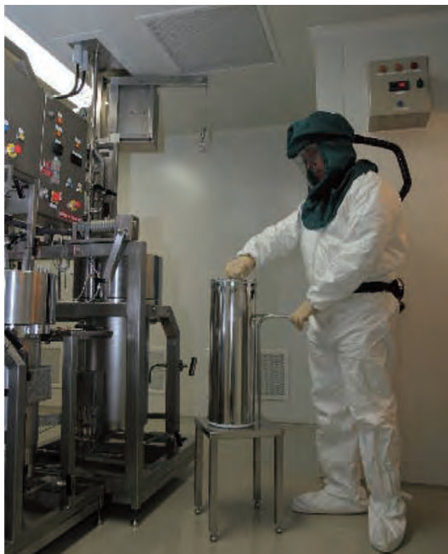
Figure 2. SCF - processed powder from a particle-generation SCF equipment harvesting in a laminar hood inside a clean room. (Courtesy SEPAREX)
