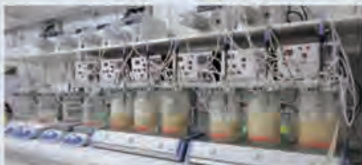
A simulated human gut – in SATIN the SHIME® model was enlarged by one step
