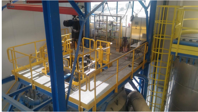
3x350 kW PCD burners in the top of the drying chamber
