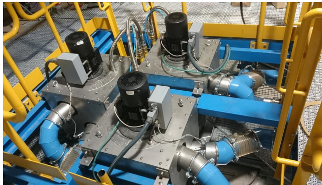
3x350 kW PCD burners in the top of the drying chamber
