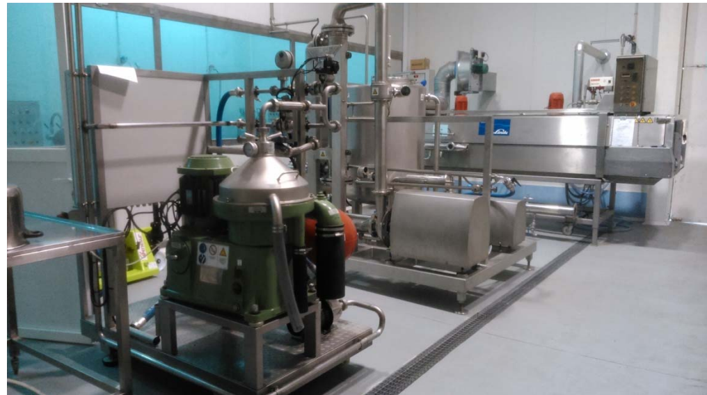
Centrifuge / Tangential filtration / Freezing tunnel
