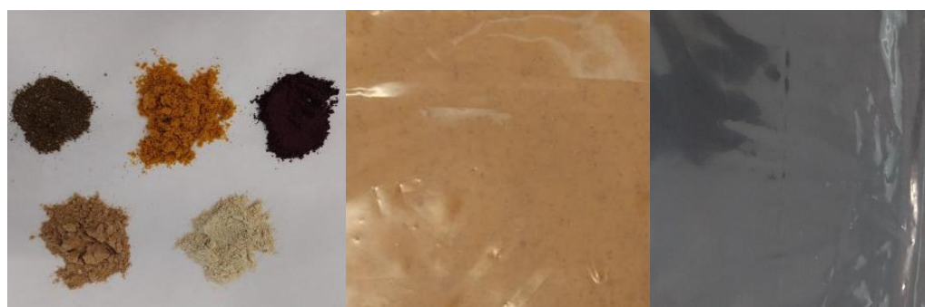
Insoluble fibers provided by UCP and CTNC (on the left), plates obtained by reprocessing in a hydraulic press (in the middle and on the right).
